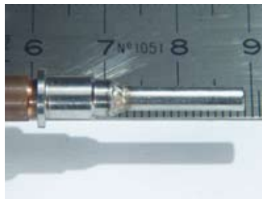
Steel 1.4021, pipe + flange gastight welding
