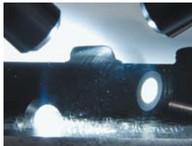
Build-up welding free from cavities
